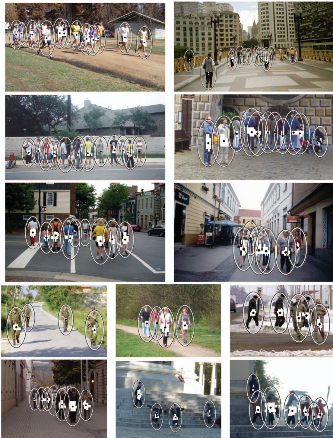
Fig. 16. Detection examples. The classifier is trained on the INRIA data set. White dots show all the detection results. Black dots are the modes generated by mean shift smoothing, and the ellipses are average detection window sizes. There are extremely few false positives and negatives.
